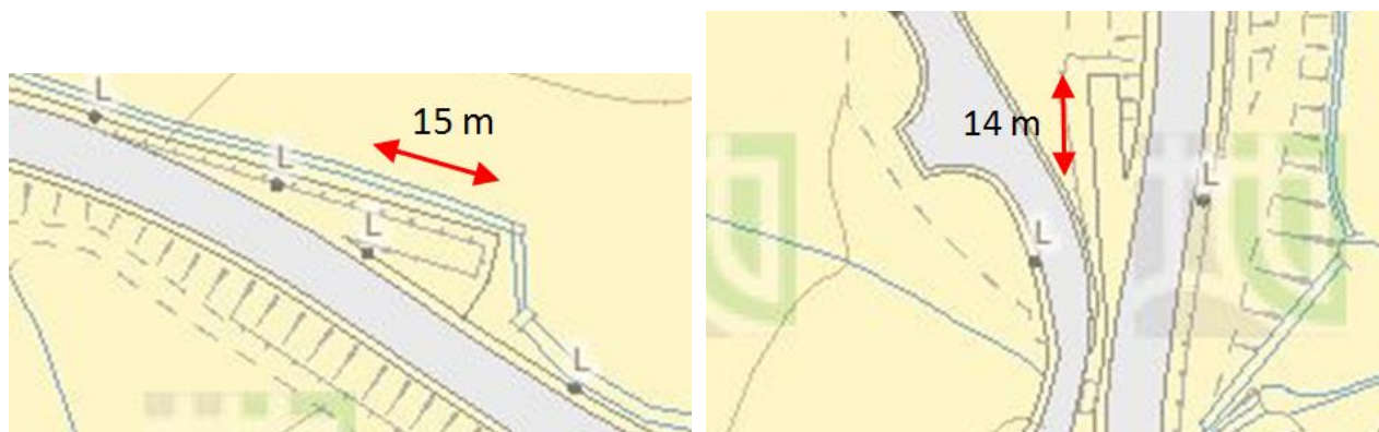
Layout and Dimensions of Arrester Bed for Southbound Traffic (left) and Northbound Traffic (right) (source of map: Lands Department)
