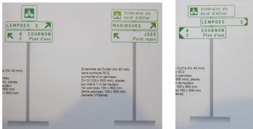
Example of bicycle directional signs with hierarchy based on upper case and italic fonts
