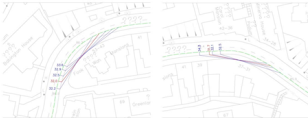
Diagram 1 Sightlines at Bends on Lyttelton Road
