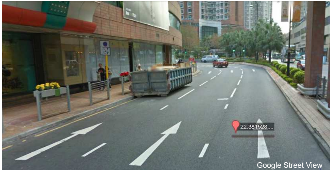
A tipper with no reflective markers directly placed on the traffic lane of a distributor road
